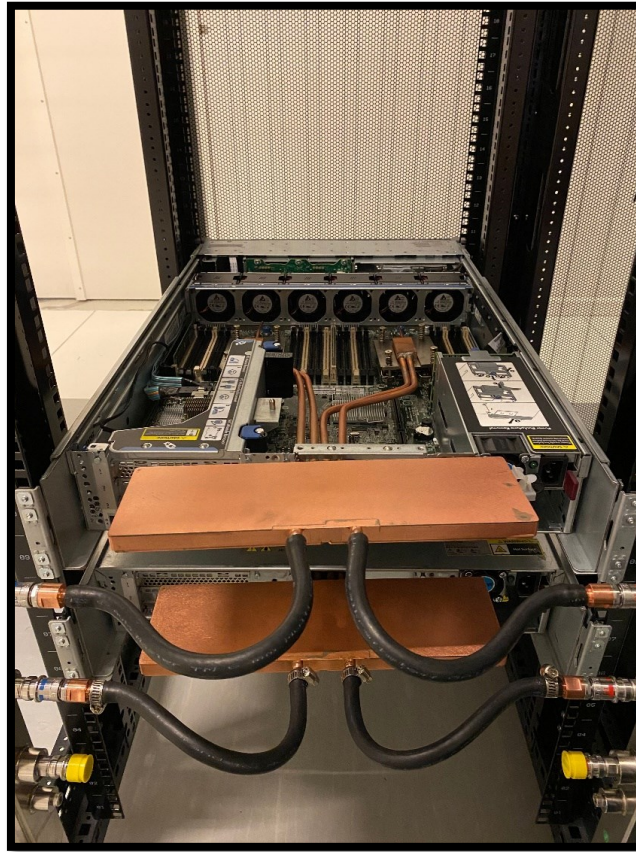
Figure 9 – Inside view of the CPU cooling configuration and connection to the heat exchanger.
